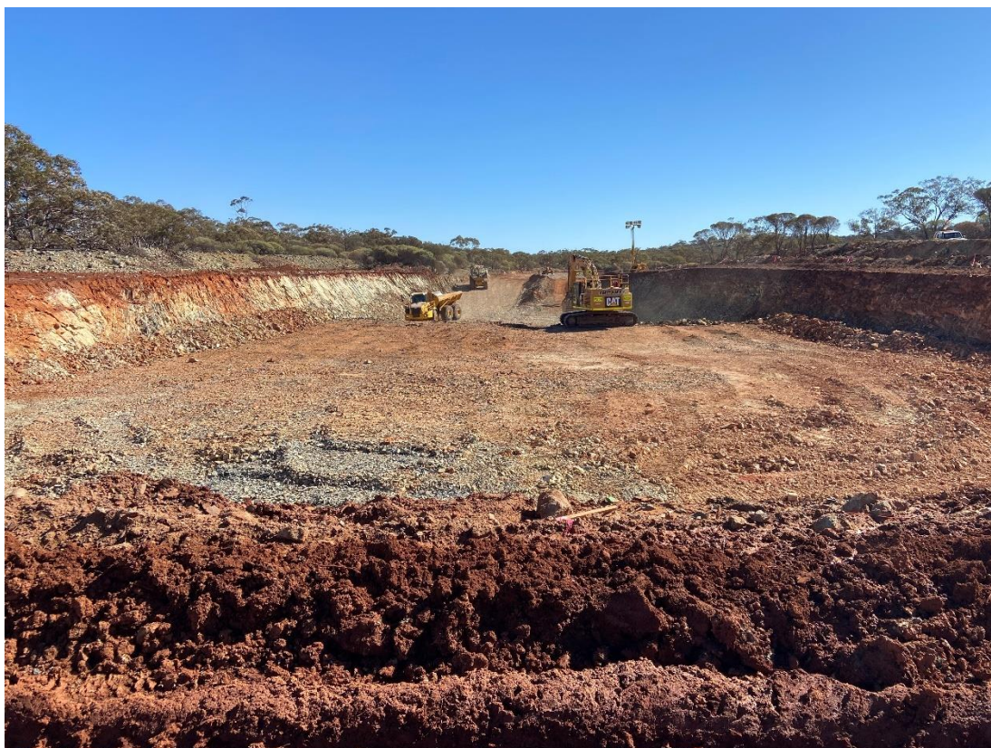
Figure 4: Rothsay boxcut excavation underway
