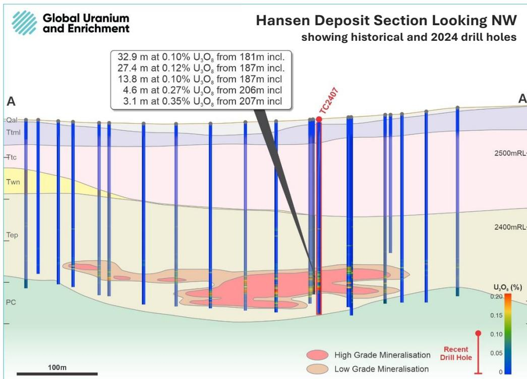
**Figure 3:** Cross Section A-A' showing results of TC2407 and TC2408 relative to historical drill holes, modelled mineralisation, and the geologic formations.
