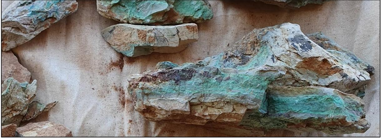
*Photo 1. Rock chip sample KB03113, which returned 15.3% Copper, comprised of oxidised white meta-tuffaceous siltstone with oxide copper mineralisation (green/dark grey in photo).*
