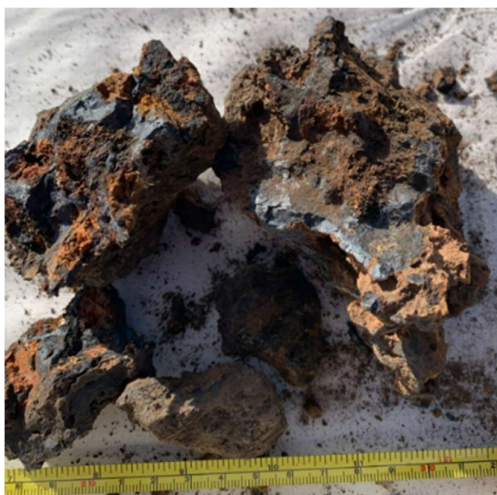
Sample GRR116 41.4% Mn, Secondary MnO, massive MnO encasing pockets/cavities of clay
