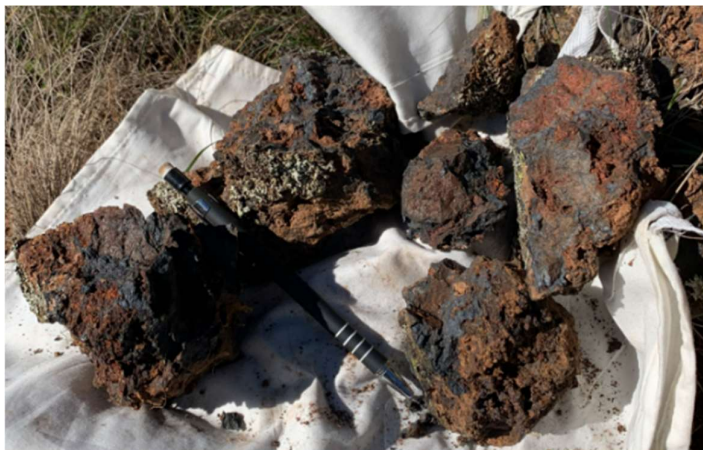
Sample GRR256 48.9% Mn Outcrop Exposure 1.2 metres x 1 metre with abundant black MnO. Sparse floaters similar up hill and down track, a large heavy block of MnO 44cmx32cm.
