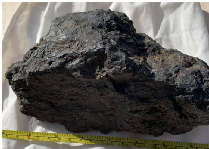
Sample GRR117 50.3% Mn, Massive MnO with minor chert, some mammillated, botryoidal textures
