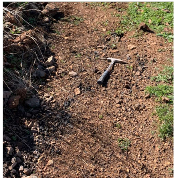
Outcrop location of sample GRR255 41.6% Mn. Outcrop on bulldozed track, exposed lode with abundant massive MnO, strike 55°-235°. Location of planned drill hole.
