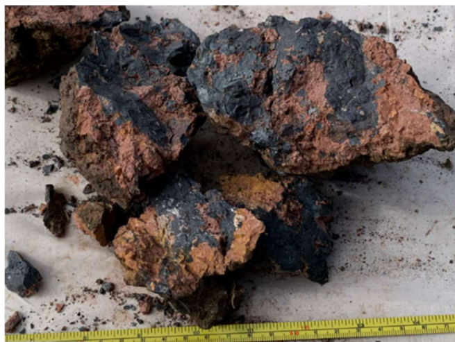
Sample GRR249 34.3% Mn, Weathered red chert with abundant clumps/clots of MnO and bands of MnO up to 5mm wide
