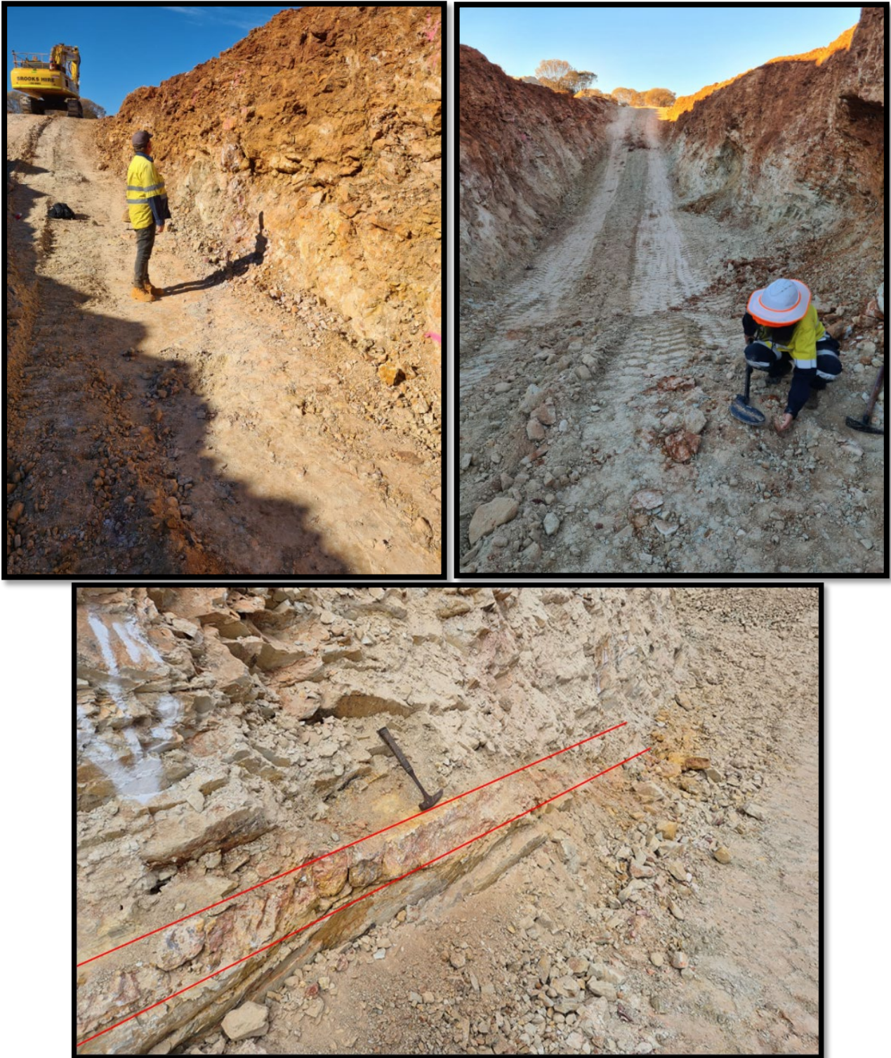
Figure 3: Revere Reef striking across ramp, highly mineralised zone in iron rich reef (4m bench floor), top. High grade reef dipping towards ramp floor reef (5m bench floor), bottom
