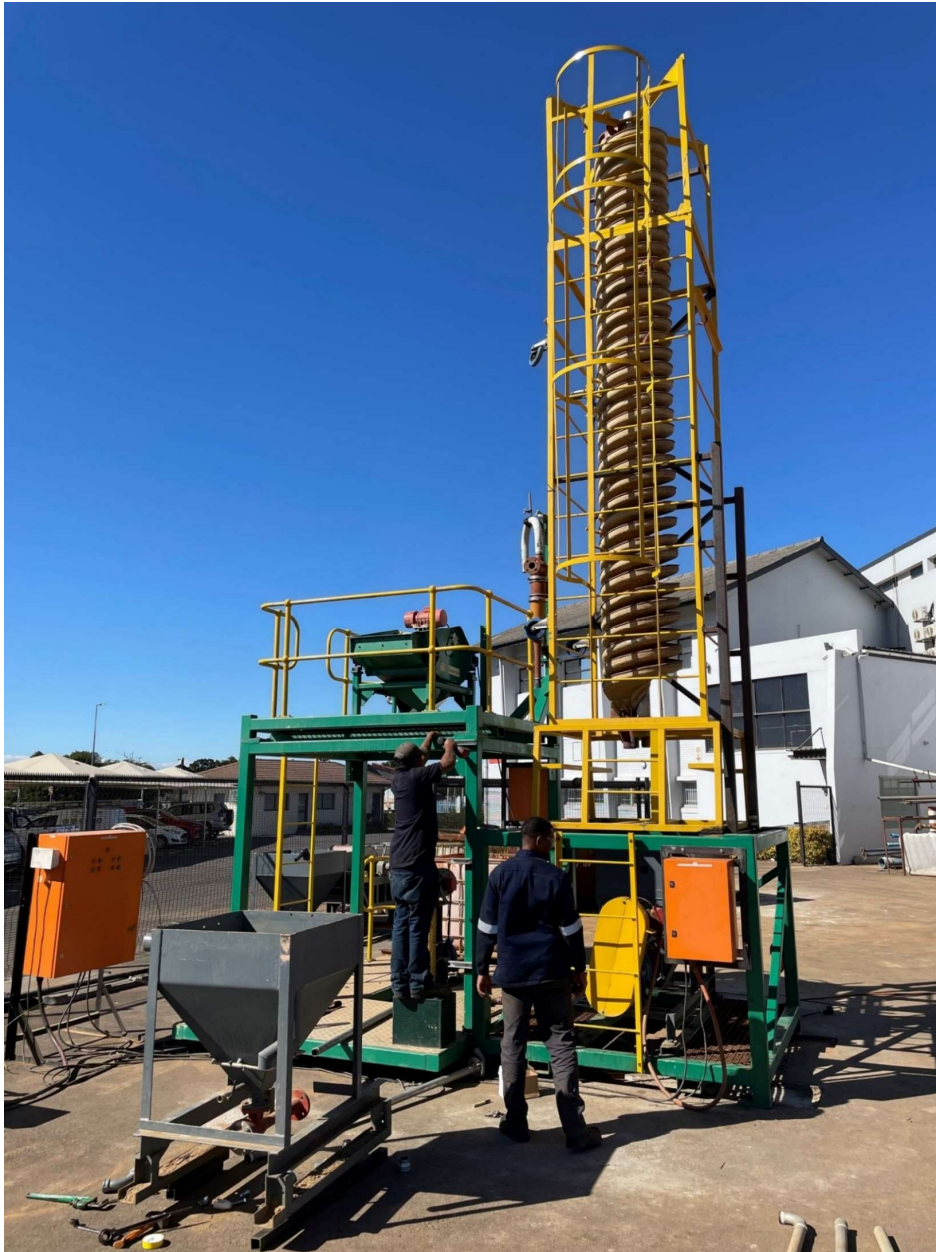
Figure 6: Final stages of assembling the spiral plant at Paterson & Cooke, South Africa
