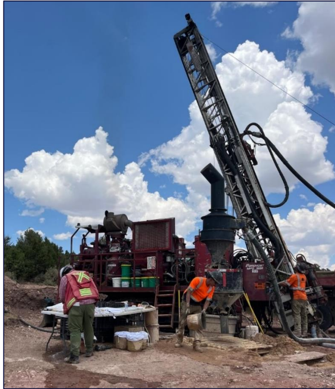
Figure 4 - Drilling Activities at Maverick Springs including pXRF of drilling material.
