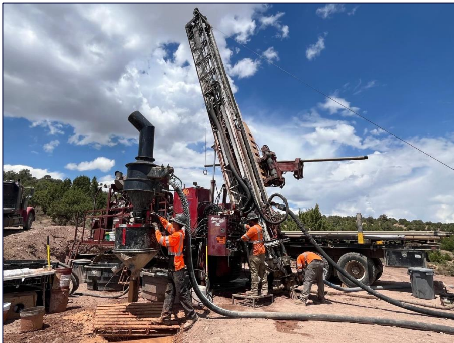
Figure 3 - Alford Drilling RC Rig at Maverick Springs.
