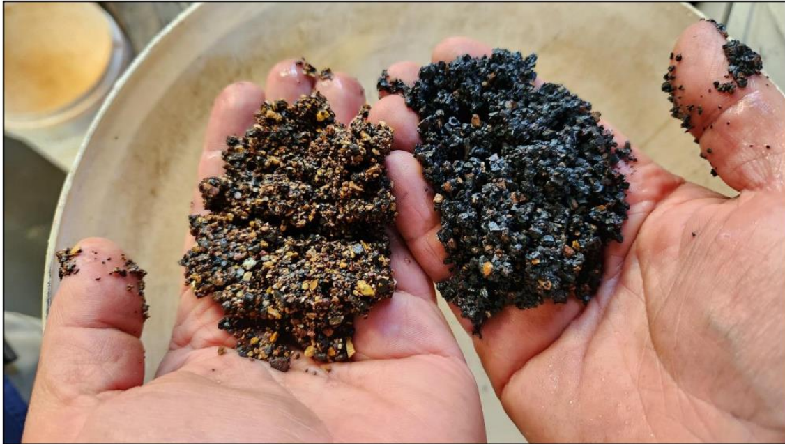
Figure 5: DMS separated material from KR2 showing beneficiated manganese ore on the right side and waste to the left.
