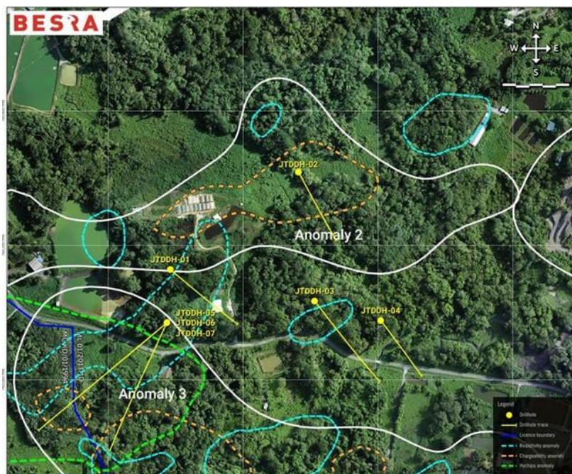
Figure 10 - 2023-2024 Exploration DDH Program. Chargeability (red polygons) and Resistivity (blue polygons). HyChips anomaly (yellow polygon) and 450hz DIGHEM resistor (dashed orange outline).
