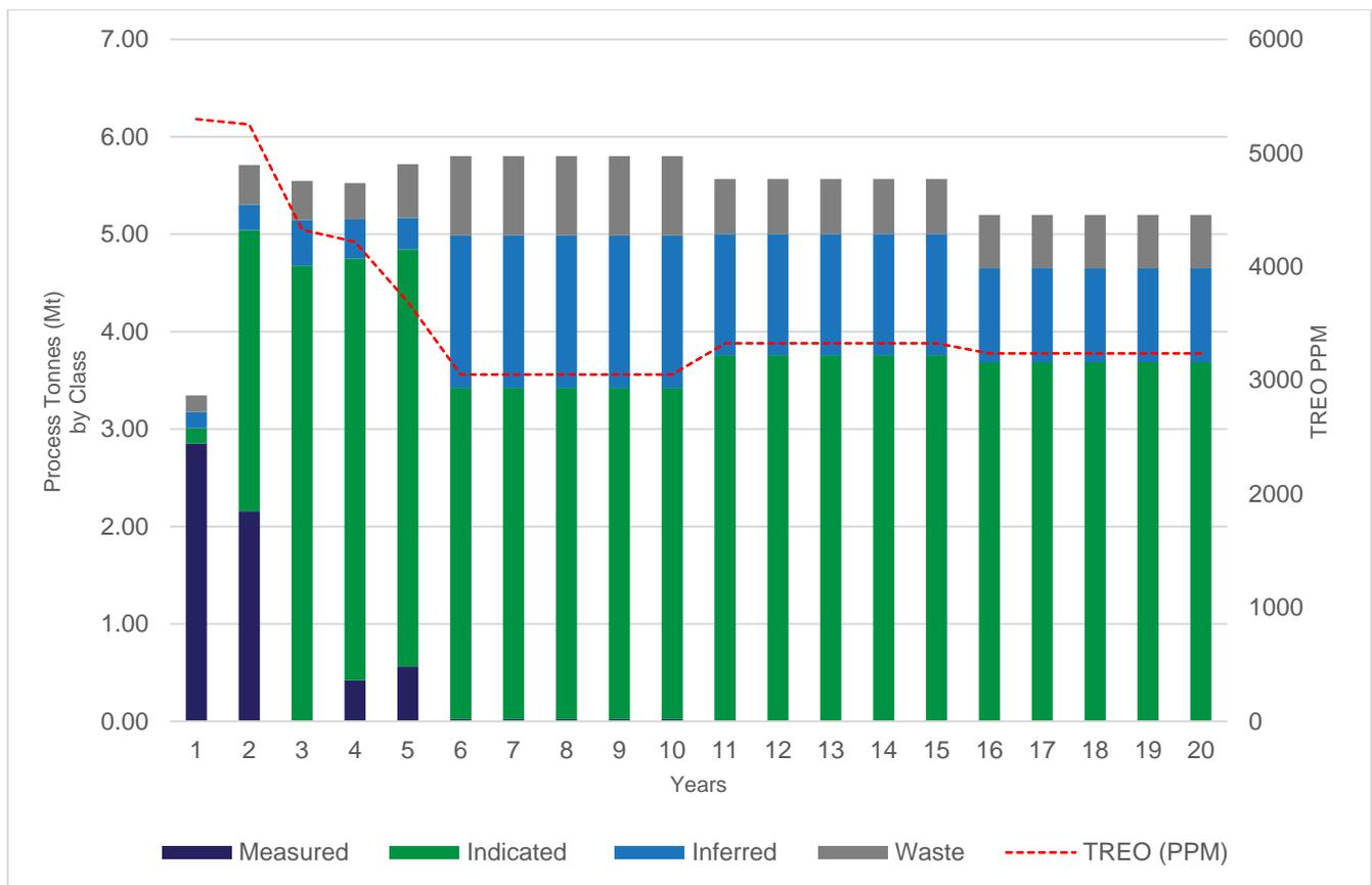
Figure 8: Mined tonnes and grade by classification
