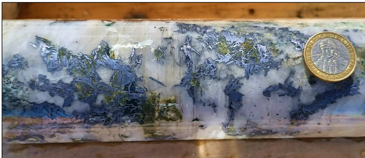
Figure 2: Example of high-grade molybdenum mineralisation in hole CMLCD014, 4,350ppm Mo (1.70% CuEq) (498m to 500m).
