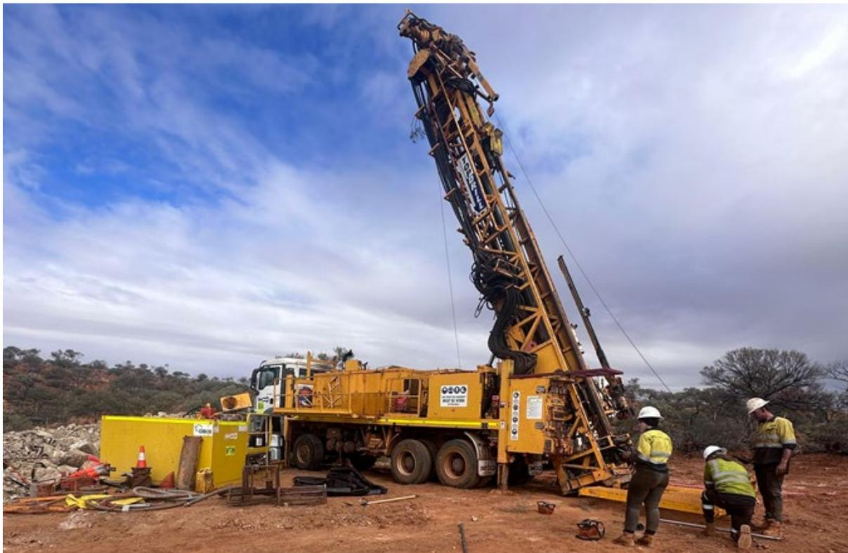
**Figure 1:** Setting-up for diamond drilling at Graphite Bull, 8<sup>th</sup> July 2024.
