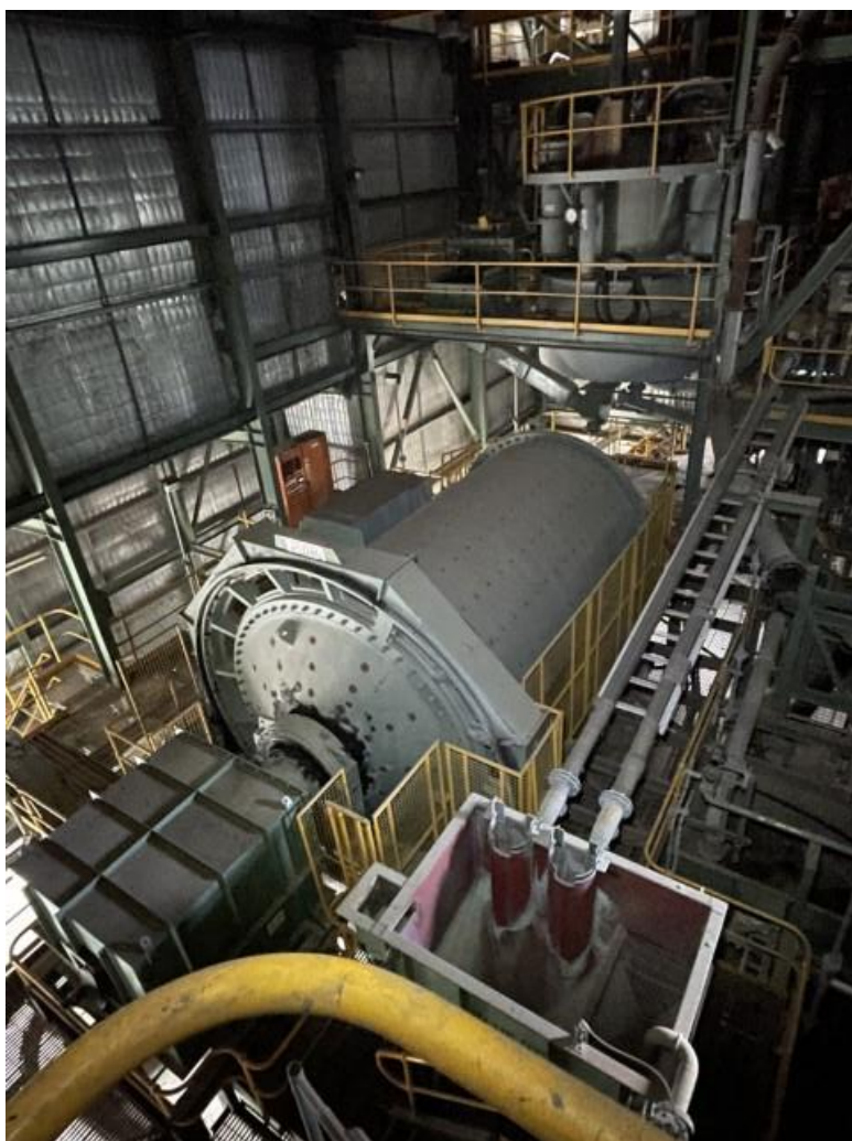
Figure 2: 750kW Outokumpu ball mill (April 2024) prior to being transported to the Murchison Gold Project.
