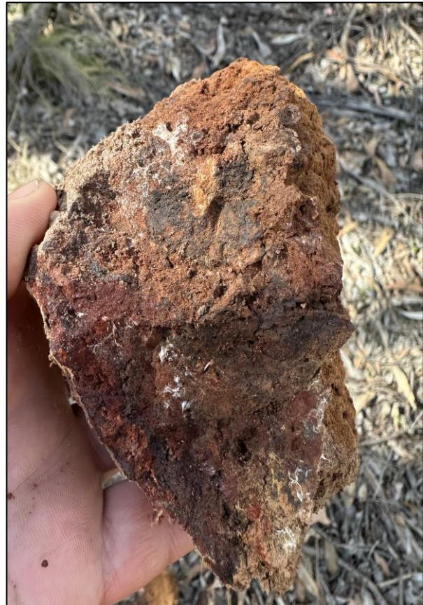
Figure 7 – Silver-Base metal mineralisation within gossan yielding 36.8 g/t Ag, 0.3% Cu-Pb-Zn & 0.2% Ba from sample 3000766
