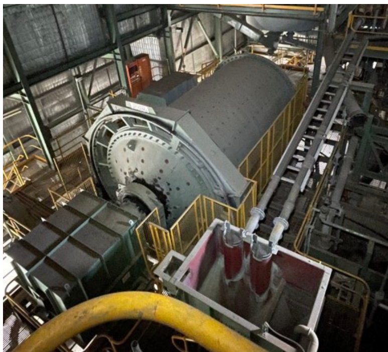
Figure 1: 750kW Outokumpu ball mill (April 2024) prior to being transported to the Murchison.
