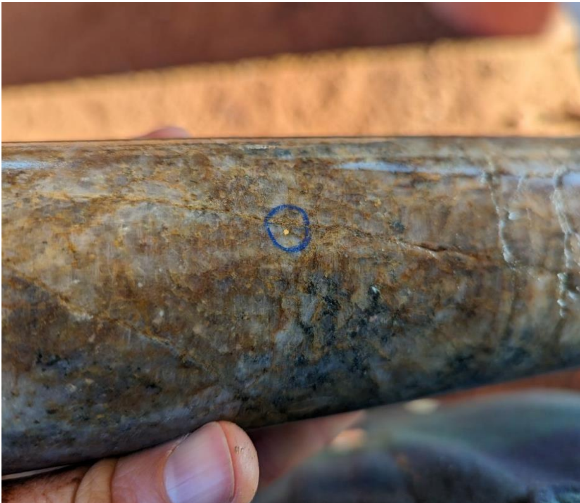
Figure 5: Image of visible gold SOMDD001 (~17.0-17.1m) where the hole assayed 1.4m @ 87.9 g/t Au from 16m. Field of view is ~8cm.
