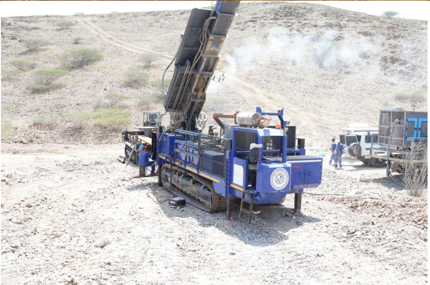
Figure 3: RC Drilling at Muvero.
