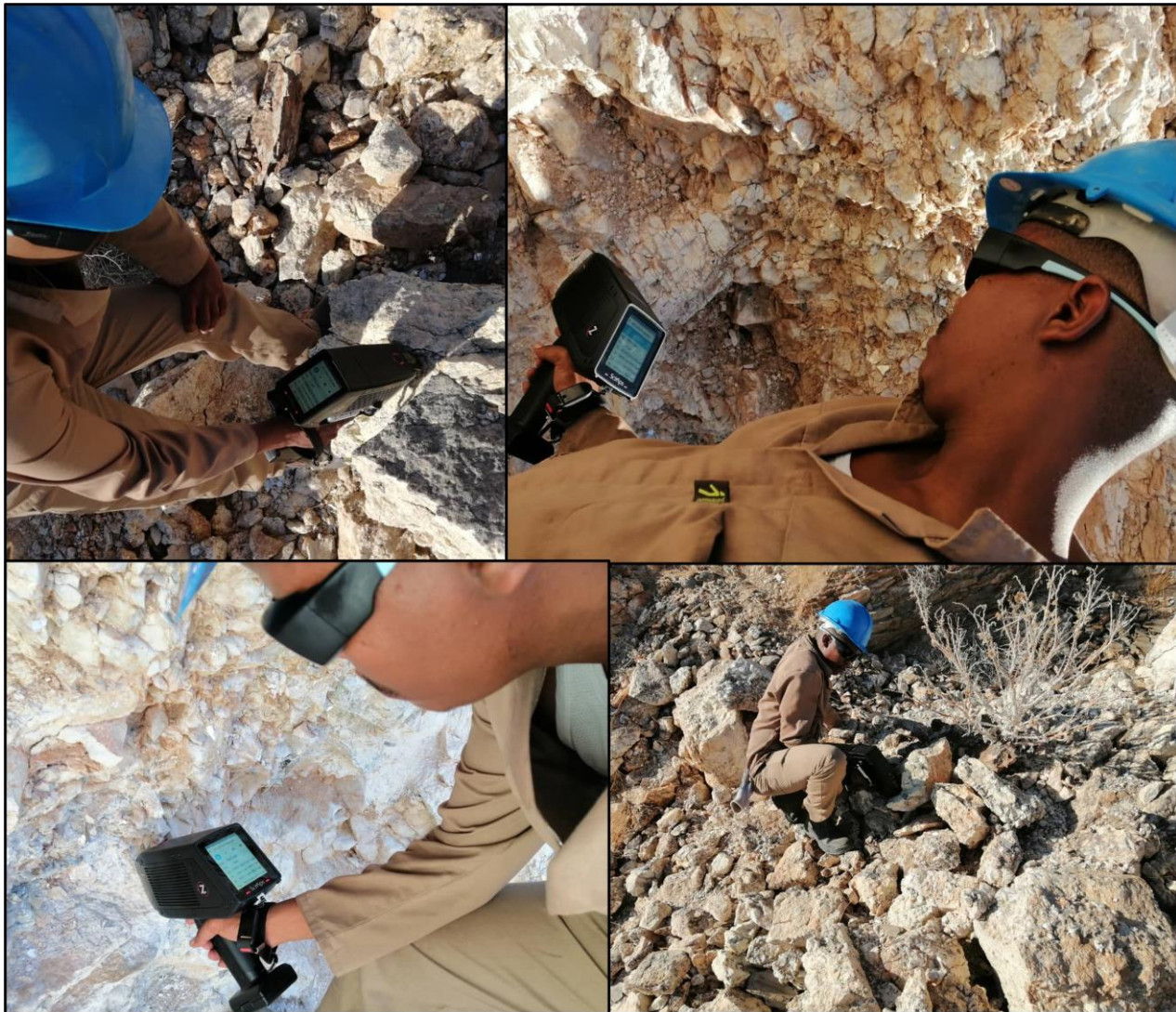
Figure 6: Handheld LIBs (Laser-Induced Breakdown Spectroscopy) instrument used in the field. Here, the team assess the potential of our pegmatite targets using the LIBS to analyse for light elements (Li, Be, Mg and B).
