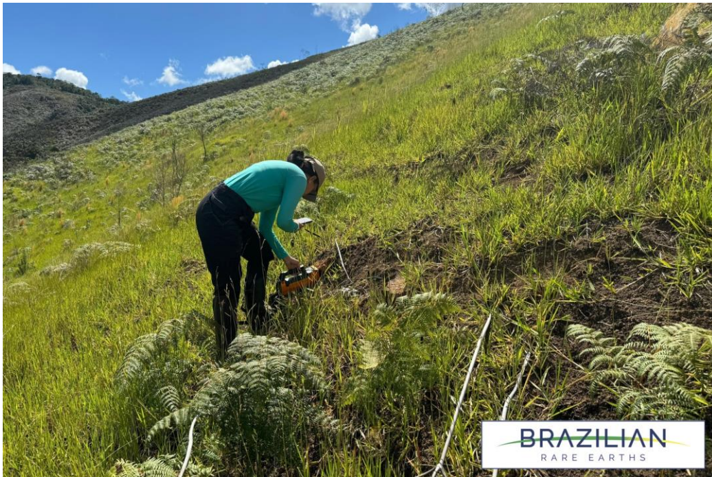
Figure 6: BRE geophysics team conducting gamma spectrometry on hard rock outcrops surrounding auger hole JEQ_CA_AUG00007
