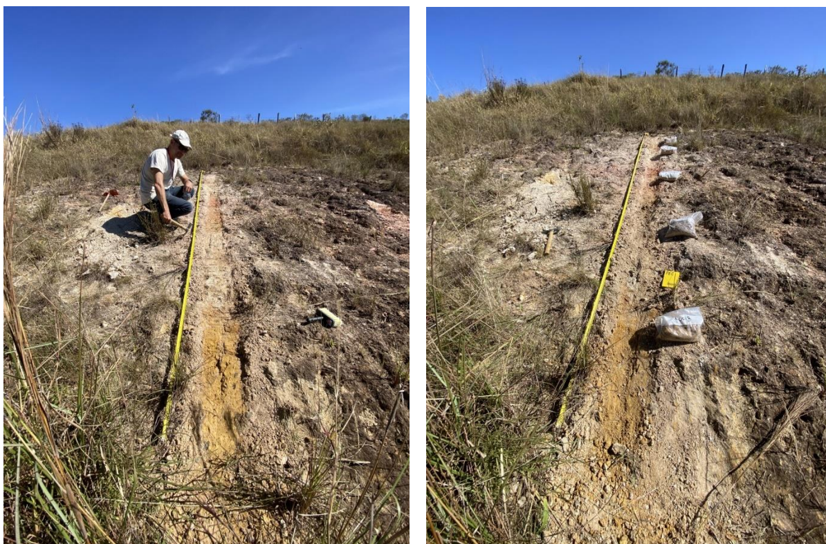
Figure 2 – Surface sampling of saprolite, with sample locations chosen after utilisation of pXRF. The 5m channel was sampled on 1m intervals, assay results are awaited.
