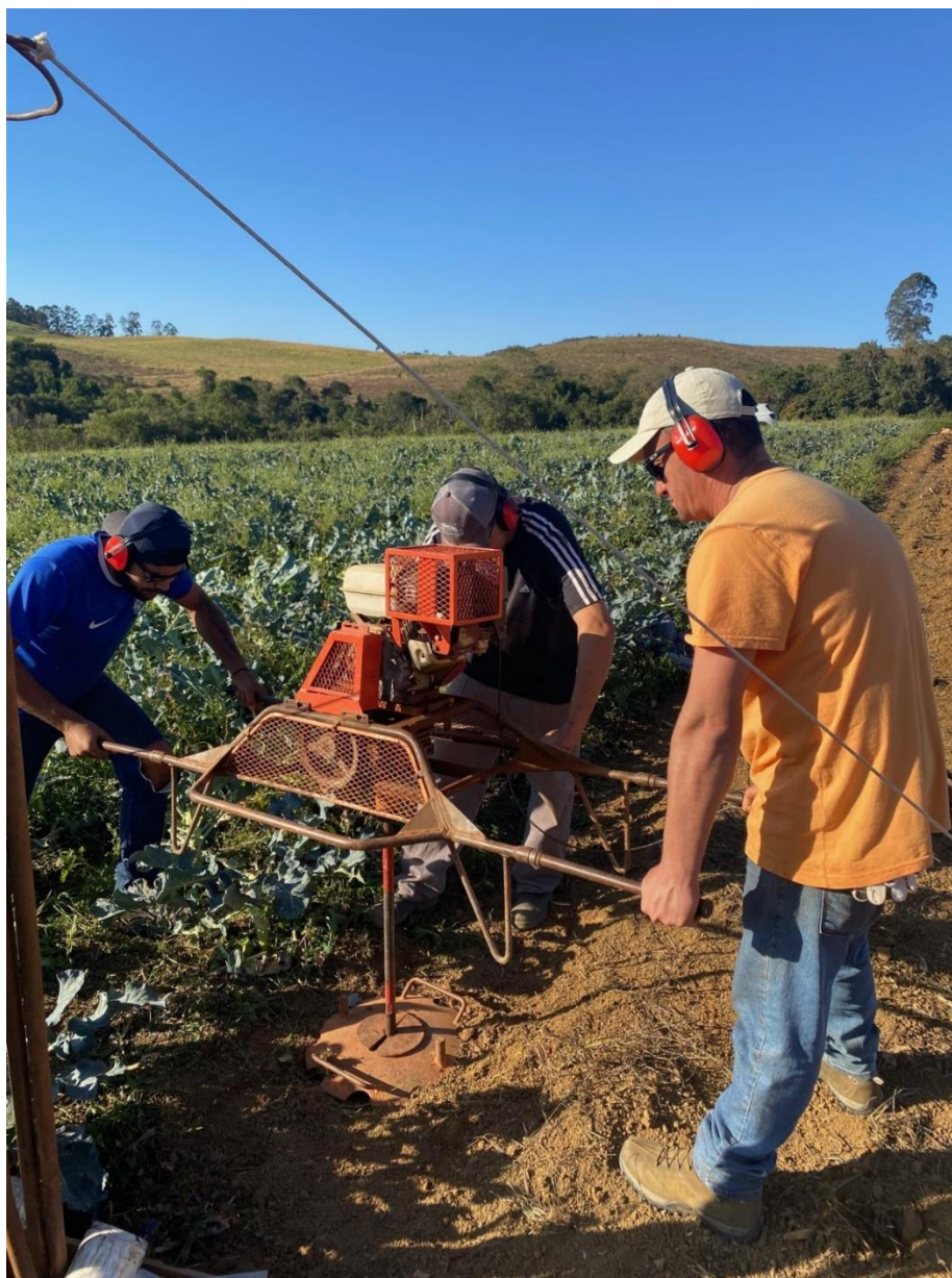
Figure 1 – Augur drilling at Perpetual's Raptor REE Project.
