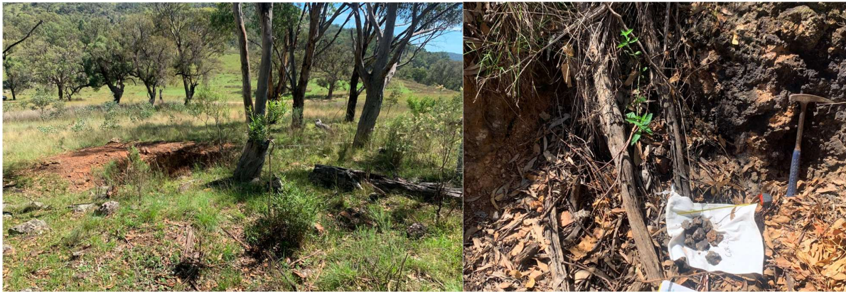
Figure 2 : Junior South trench (LHS photo) where rock samples GRR230 (47.62% Mn) and GRR231 (50.88%Mn) were taken field checking geophysical anomaly TMM02. Sample GRR231 was collected from outcrop in the wall of the trench (RHS photo).
