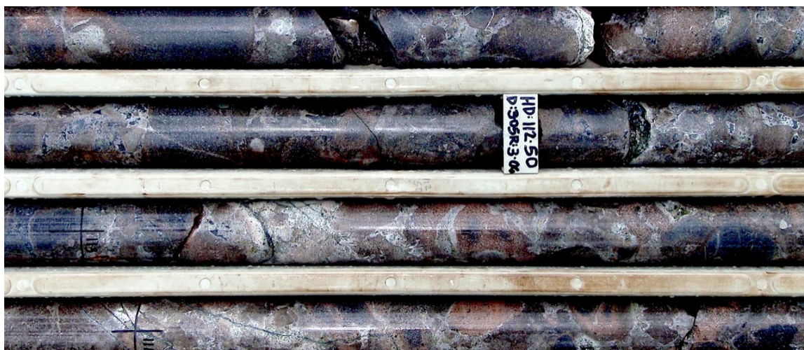
Figure 3 - Close up core photo from previous drill hole SBDD0003 (Geopacific HQ, 111.2m to 114.70m) illustrating jigsaw crackle breccia, clast supported with infill of quartz and sulphides.
