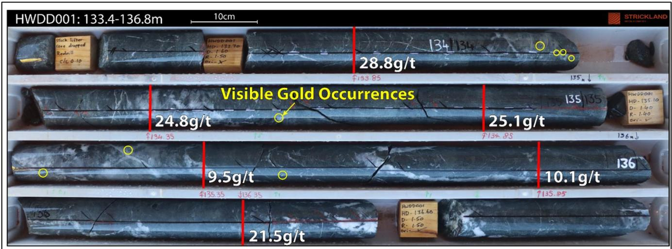
**Figure 2 (iii) HWDD001 Core Tray # 59: Visible gold occurrences (yellow circles) in relation to the received Au gold grades (white text). Sample intervals are flagged as red vertical lines.**
