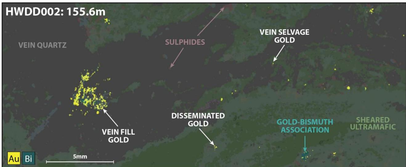
**Figure 3: Micro XRF analysis of HWDD002 drill core at 155.6 metres. Occurrences of visible gold (yellow) in relation to bismuth, veining and sheared ultramafic host lithology.**
