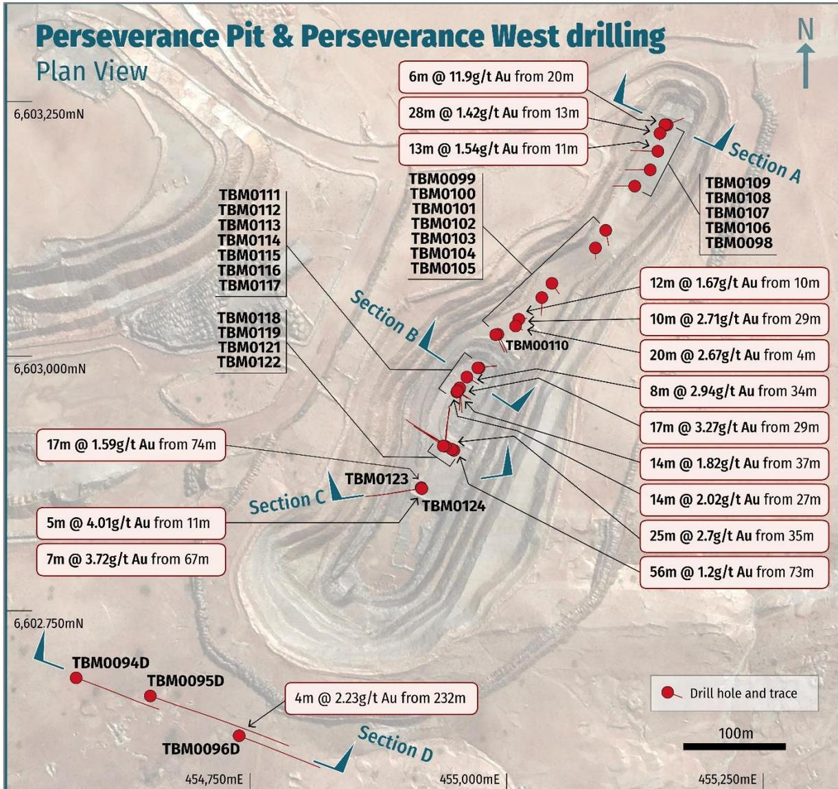
Fig 2 – Perseverance Mine with new drill collar locations, key intercepts and section lines
