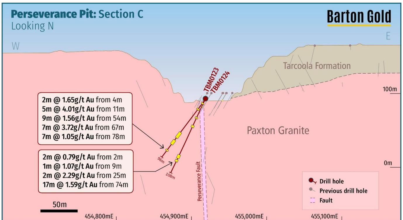
**Fig 4 (Section C) - Holes TBM0123 and TBM0124 in the southern area of the Perseverance open pit**
