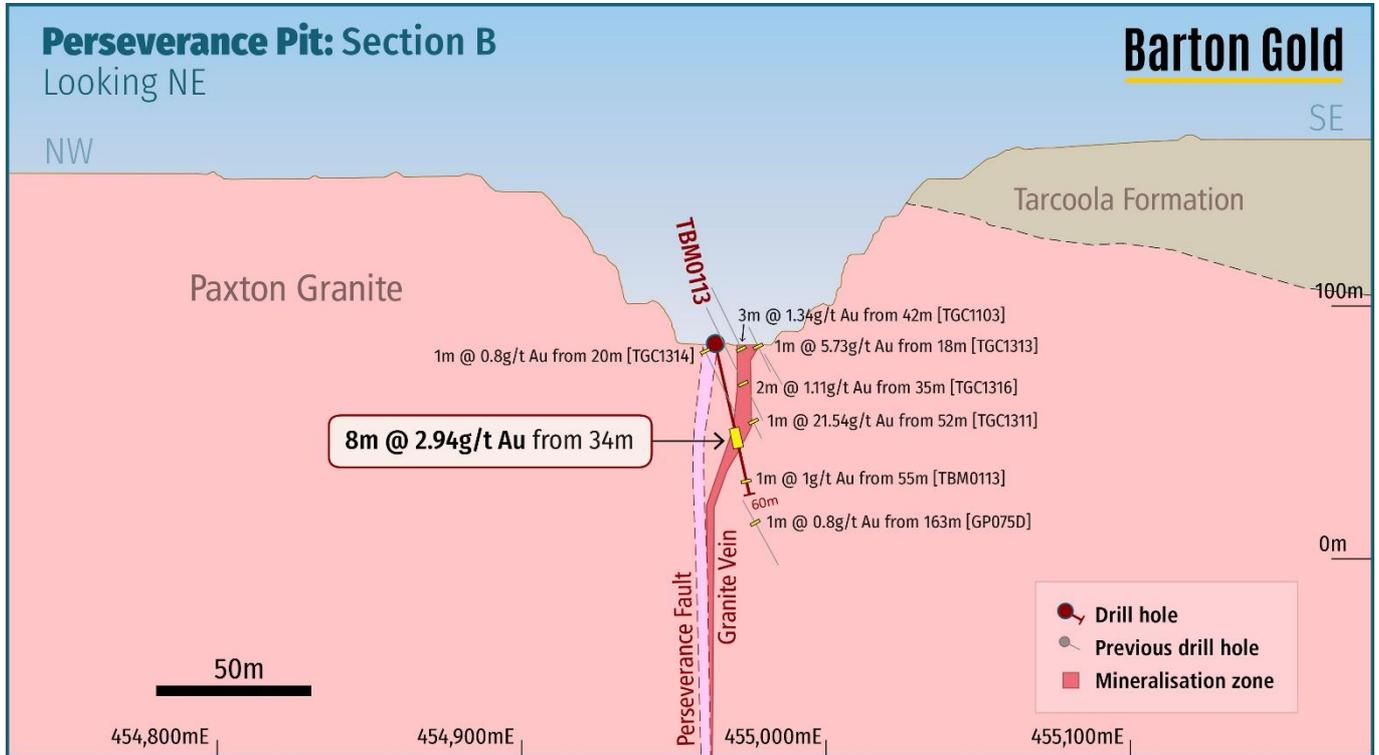
**Fig 3 (Section B) - Hole TBM0113 in the central area of the Perseverance open pit mine**
