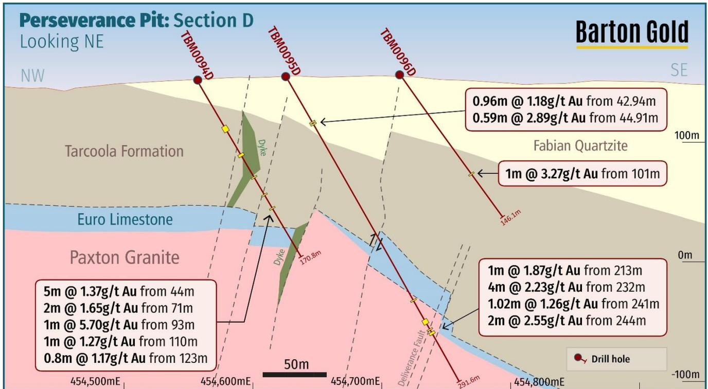
Fig 5 (Section D) – DD holes TBM94D, TBM95D & TBM96D in Perseverance West zone south of pit
