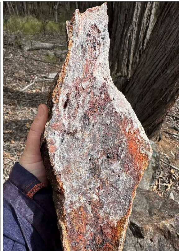
Figure 7 – Silver-Base Metal mineralisation within large baritic boulder yielding 96.7g/t Ag, 0.25% Ba 3000292
