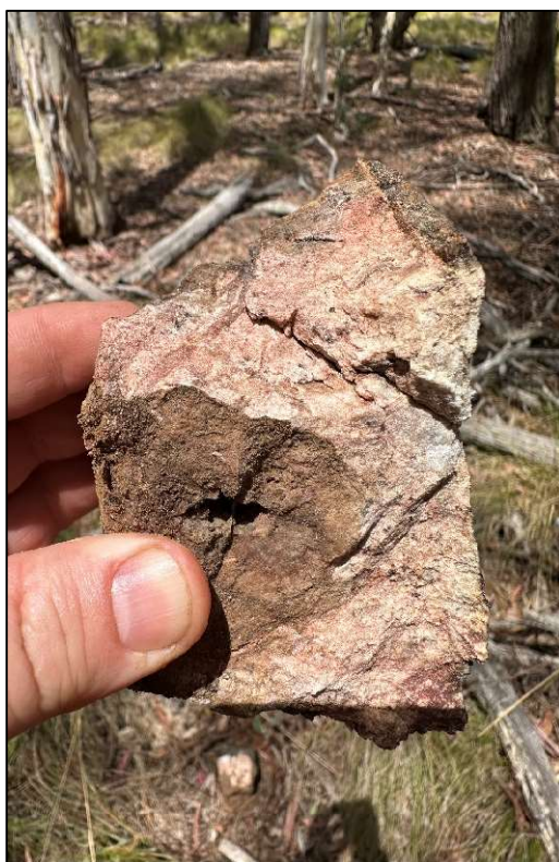
Figure 4 – Silver mineralisation within ferruginous sandstone yielding 318 g/t Ag, 0.37% Ba from sample 3000298
