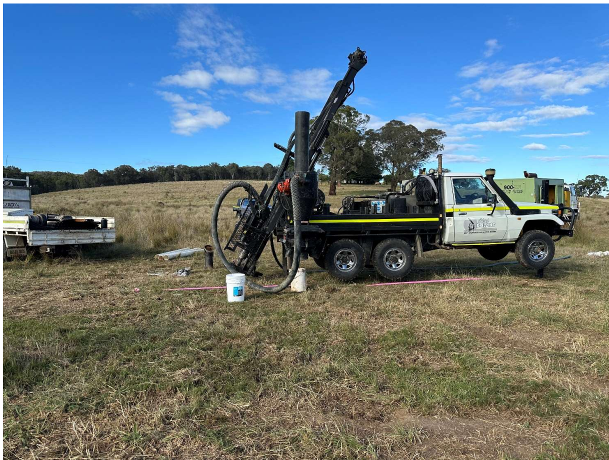
Figure 13 – RC Drill Rig commencing the drilling of the first hole
