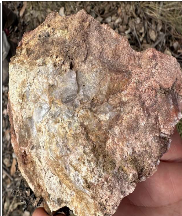
Figure 11 – Silver-Base metal mineralisation within oxidised barite yielding 115 g/t Ag from sample 300361
