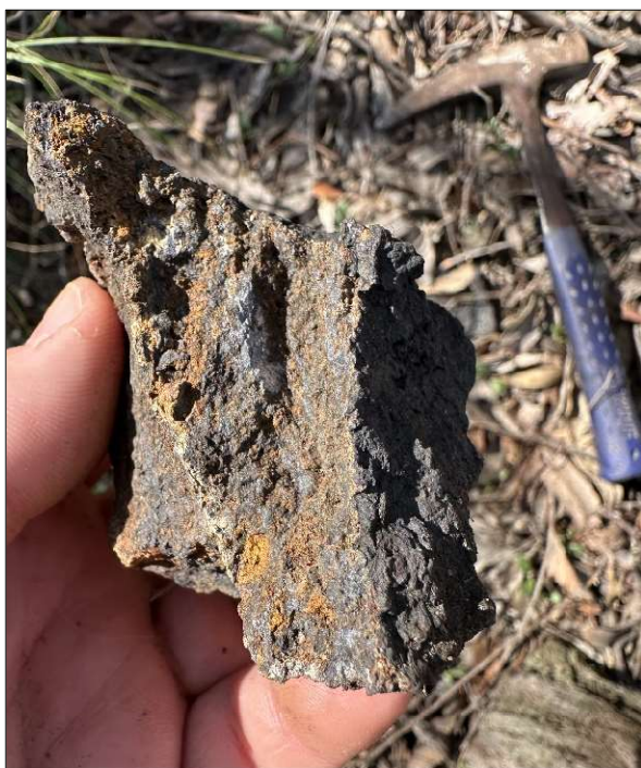
Figure 10 – Silver-Base metal mineralisation within ferruginous gossan yielding 177 g/t Ag , 2.11% Cu-Pb-Zn & >1% Ba from sample 300356
