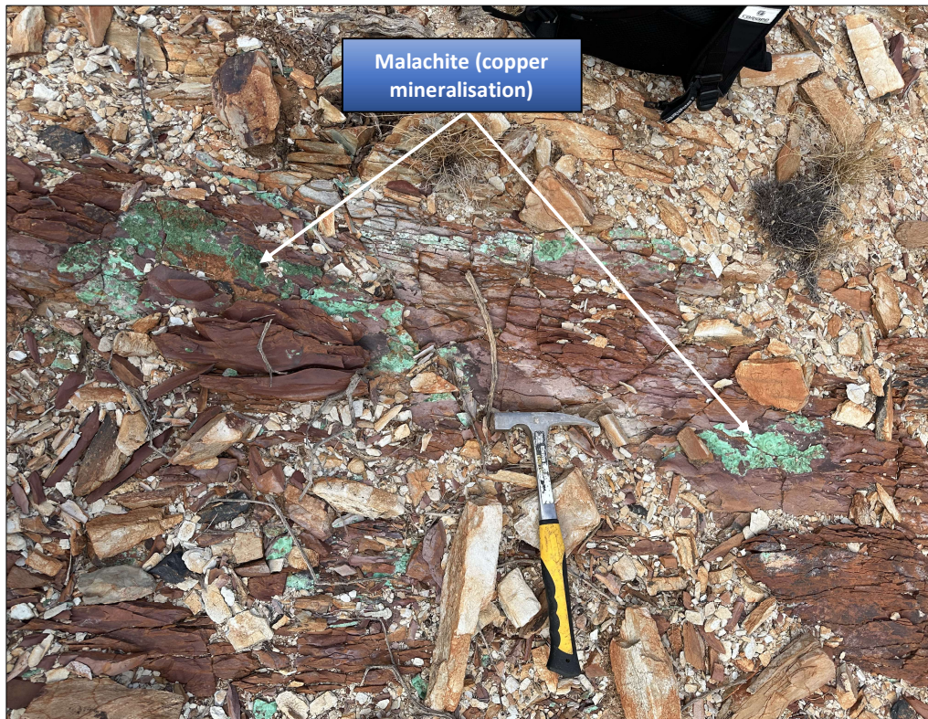
Figure 15 – Rock Chip Sample CH213 - Malachite eastern edge of 8-10m copper zone, strike 160° dip -30. Assay Results: 8.64% Cu
