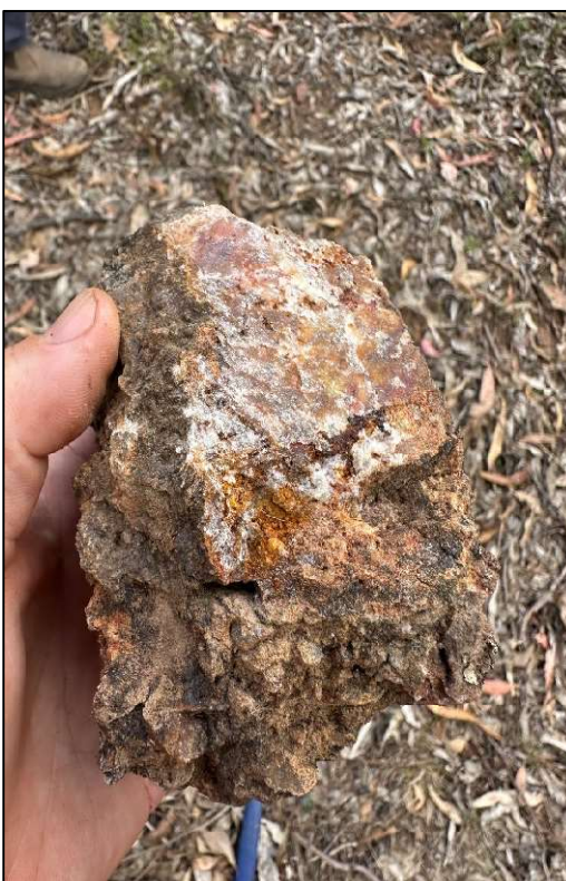
Figure 5 – Silver mineralisation within ferruginous quartz yielding 183 g/t Ag, 970 ppm Ba from sample 3000551
