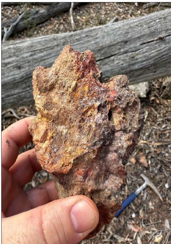
Figure 6 – Silver-Base Metal mineralisation within gossanous siltstone yielding 80.9 g/t Ag, 0.1% Cu, 0.4% Pb & 0.12% Zn, 0.51% Ba 3000287 from sample 3000551
