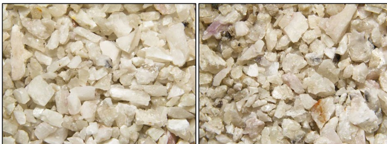
Figure 5 - HLS concentrate fractions grading ~6.0% Li 2 O (left) and ~5.5% Li 2 O (right)
