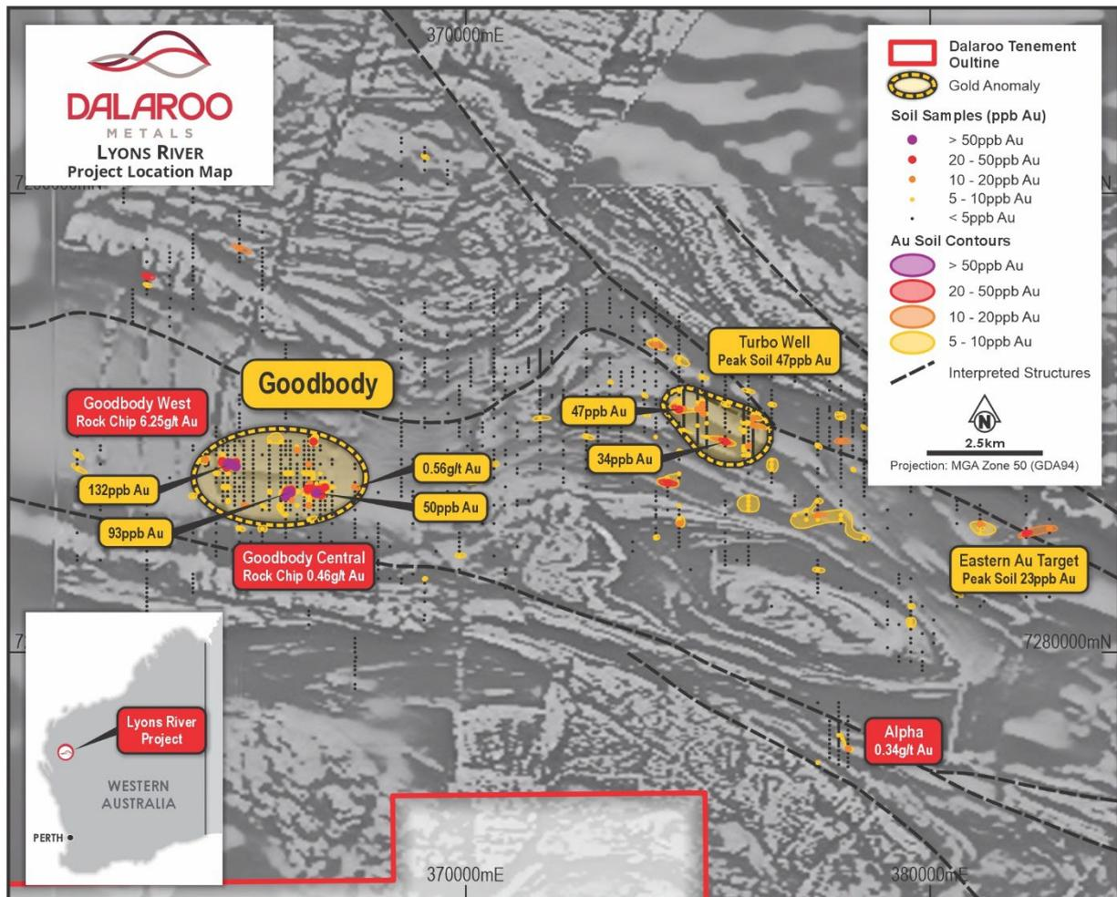
**Figure 1:** Location of Goodbody prospect in relation to additional gold prospects and interpreted regional structures within Lyons River Project area. Overlaid on greyscale Total Magnetic Intensity (TMI) 1VD base map.
