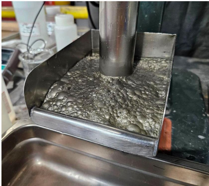
**Figure 9: 3rd cleaner sulphide concentrate assaying 29.1% nickel**
