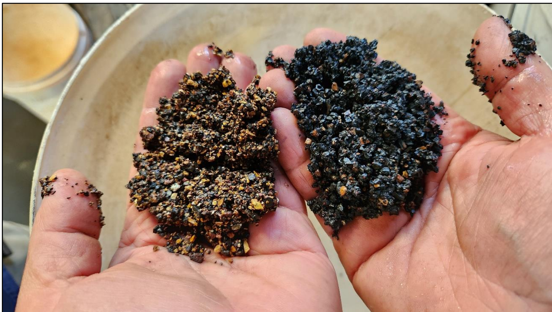
Figure 2. DMS separated material from KR2 showing beneficiated manganese ore on the right side and waste to the left.
