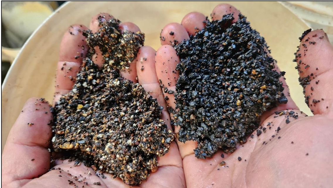
Figure 1. DMS separated material from KR1 showing beneficiated manganese ore on the right side and waste to the left.
