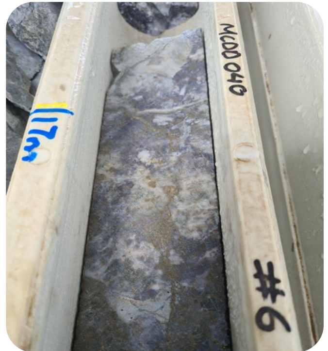
Figure 7: Drill-Core from Recent Drill Hole MCDD040 Showing Clear Brecciation and Semi-Massive Chalcopyrite Stringer.
