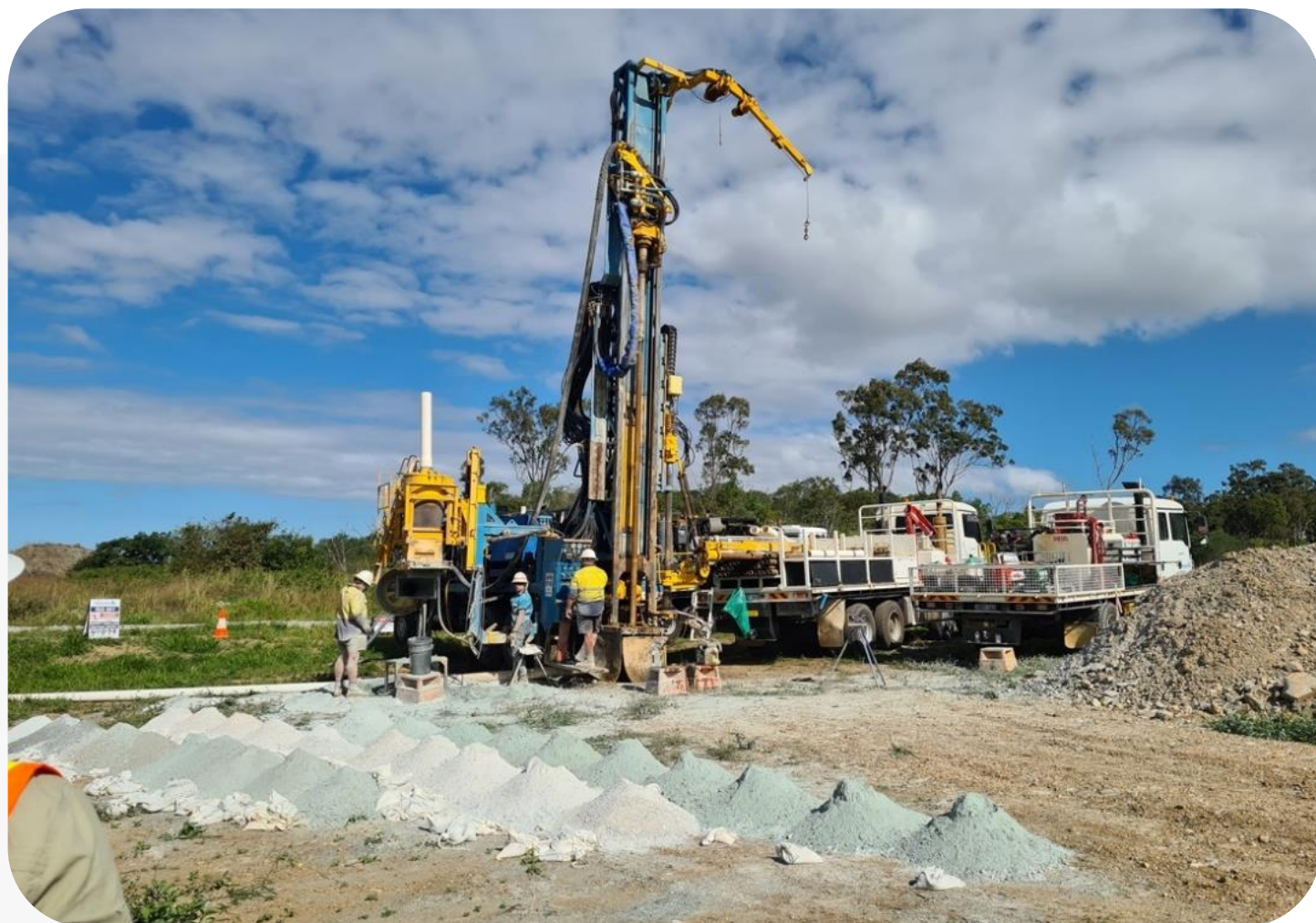
Figure 6: Q Mines RC Drilling at the Mt Chalmers project (October 2022).
