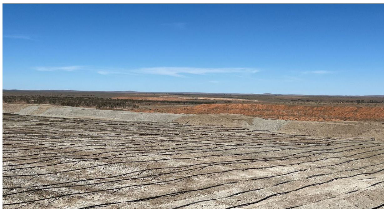
Figure 6: New Heap leach cell with leach reticulation installed.
