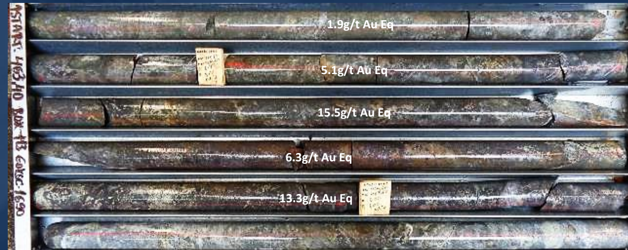
High-grade Copper-Gold mineralization in EOKSC1690 – southern end of the Shanac deposit
