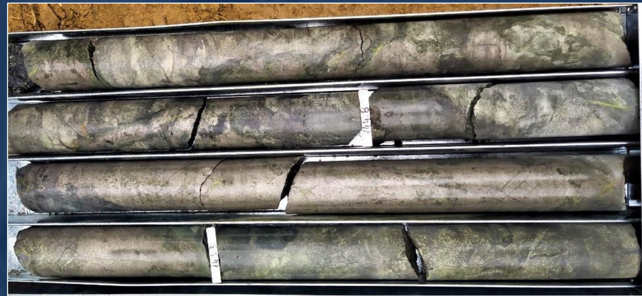
2.6g/t Au and 1.7% Cu in ZRSD20135a at Copper Canyon
