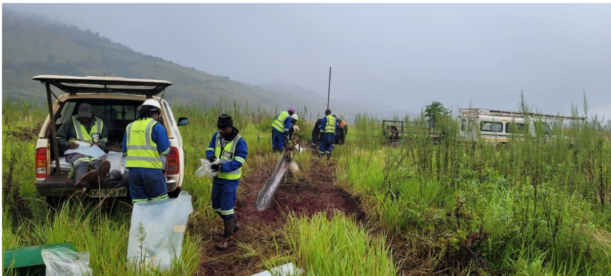
Figure 3 – Drill samples being labelled by SGS at the Blyde #2 tailing near the TGME plant
