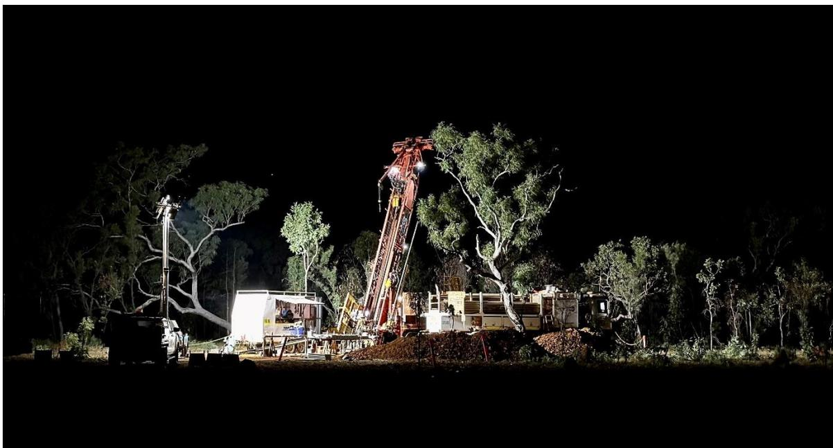
Figure 8: Image of the Topdrill diamond rig drilling at Orion.
