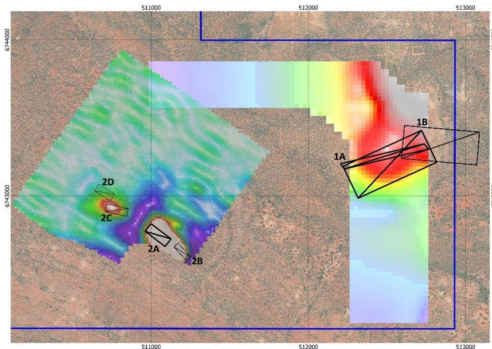
**Figure 1:** Images for Channel 36 in east (late time) and Channel 20 in the west (mid-time) showing the location of the various interpreted bedrock conductive plates (black polygons).
