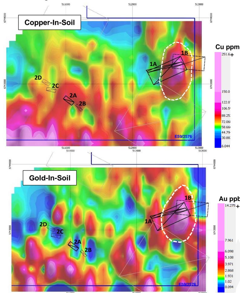
**Figure 2** (upper) colour gridded copper-in-soil image showing EM anomalies (black polygons) and coincident copper anomaly (white dash). (Lower) colour gridded gold-in-soil image showing EM anomalies (black polygons) and coincident gold anomaly (white dash).
