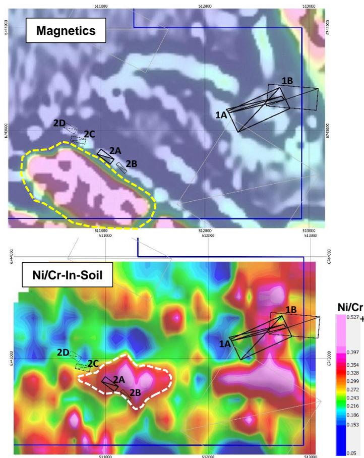
**Figure 3:** (upper) Airborne MrtpcMrtplap magnetic image showing EM anomalies (black polygons) and associated strong magnetic body (yellow dash). (Lower) colour gridded Ni/Cr-in-soil image showing EM anomalies (black polygons) and coincident Ni/Cr anomaly (white dash).
