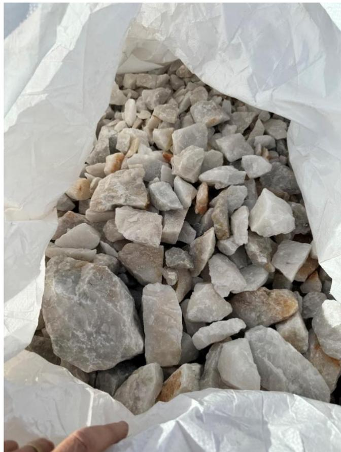
**Figure 5:** Raw quartz sample bagged ready to send to interested parties for HPQ testwork and assessment.
