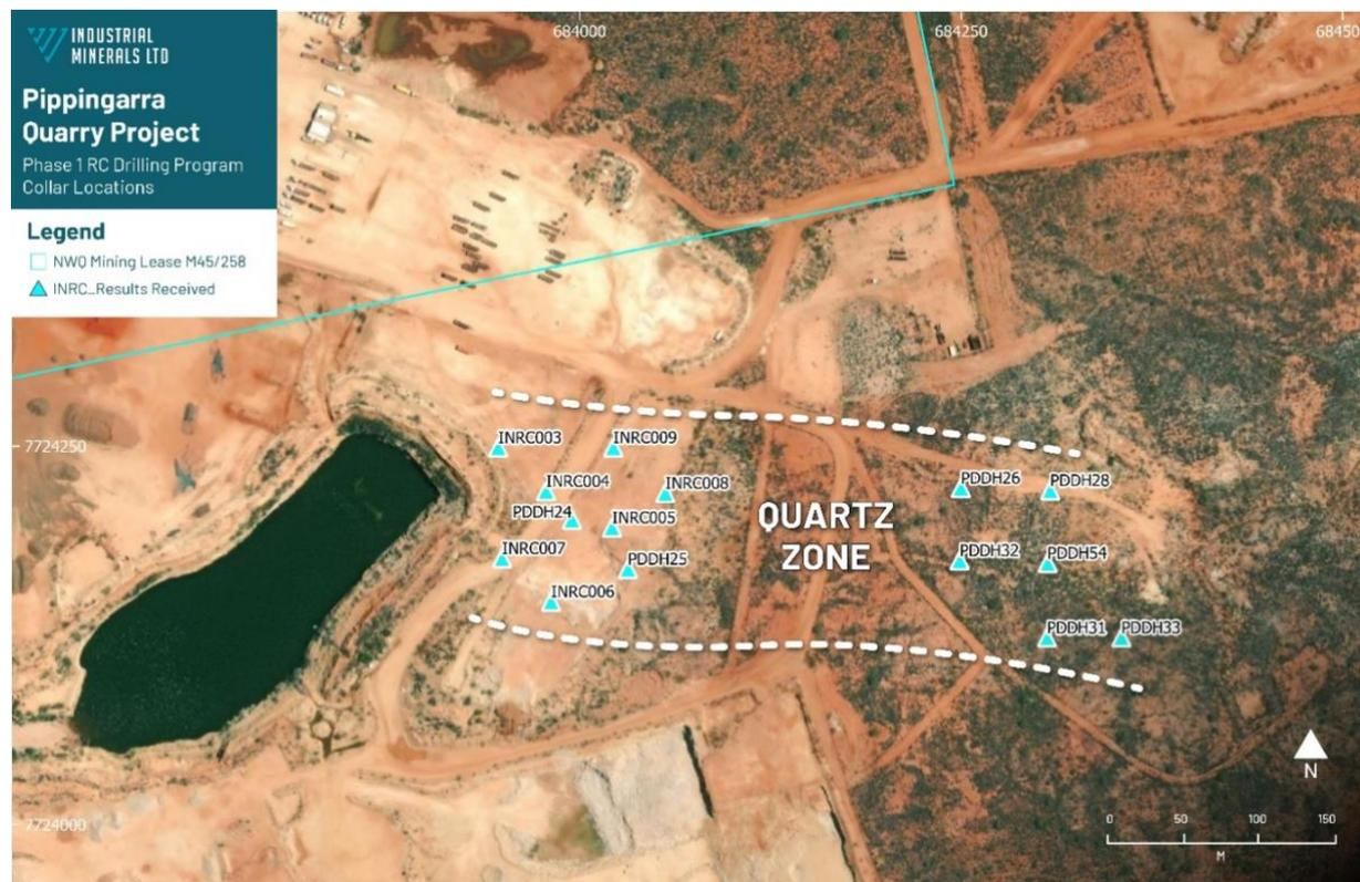
**Figure 2:** Quartz zone identified in Phase 1 RC and historical diamond drilling results.
