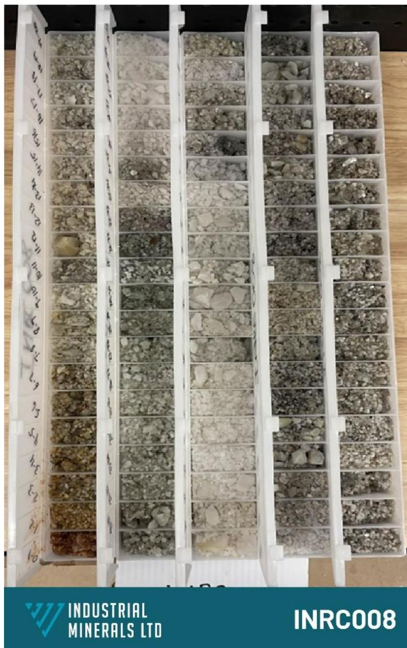
**Figure 3:** RC drill hole INRC008 - 20m white quartz intersection 35m to 55m.
