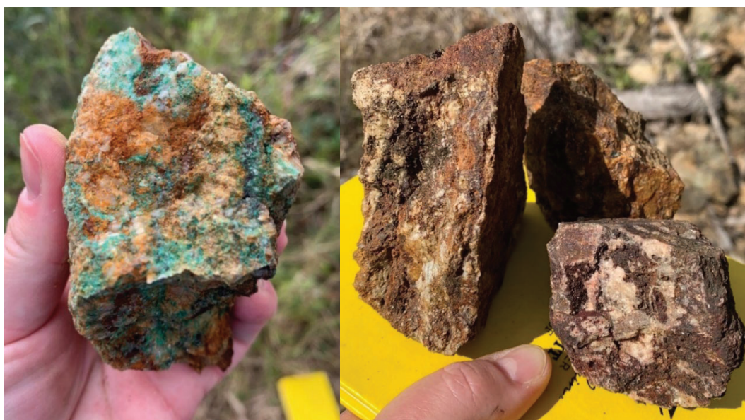
Figure 3. Sample MRRK071, 3.49g/t Au, 2.8% Cu & 195g/t Ag (left). Sample MRRK072, 6.06g/t Au, 585g/t Ag, 1.5% Cu, and 3.58% Sb (right).
