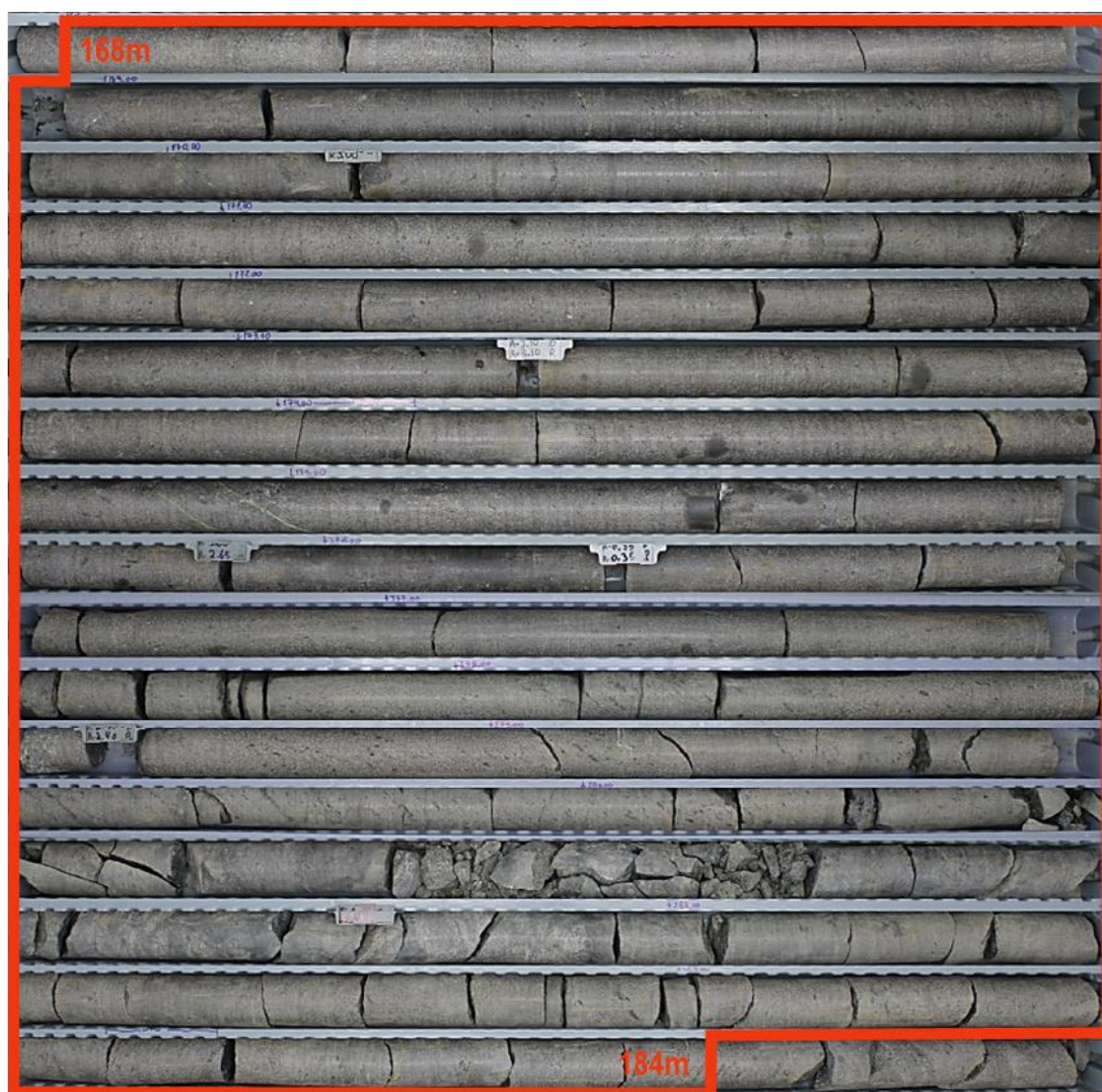
Figure 6: Diamond drill core from MADD0099: 16.0m at 29.1% TREO from 168m within 75.8m at 13.8% TREO
