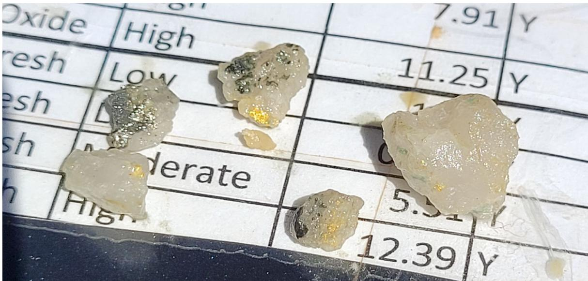
Figure 1: RC chips from 22SARC005 showing visible gold (interval 172-173m down hole).
