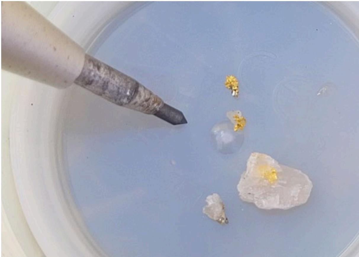
Figure 2: RC chips and visible gold panned from 22SARC005 (interval 172-173m down hole).
