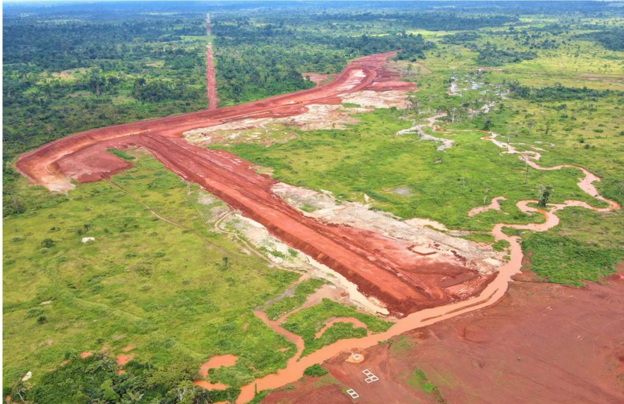
*Figure 7 Water dam and water diversion channel*
