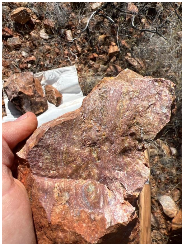
Figure 2: Massive monazite sample MWGS1108 (left) and MWGS0848 (right) which assayed 28.07% TREO with 4.63% \text{Nd}_2\text{O}_3 + \text{Pr}_6\text{O}_{11} and 23.81% TREO with 3.97% \text{Nd}_2\text{O}_3 + \text{Pr}_6\text{O}_{11} .
