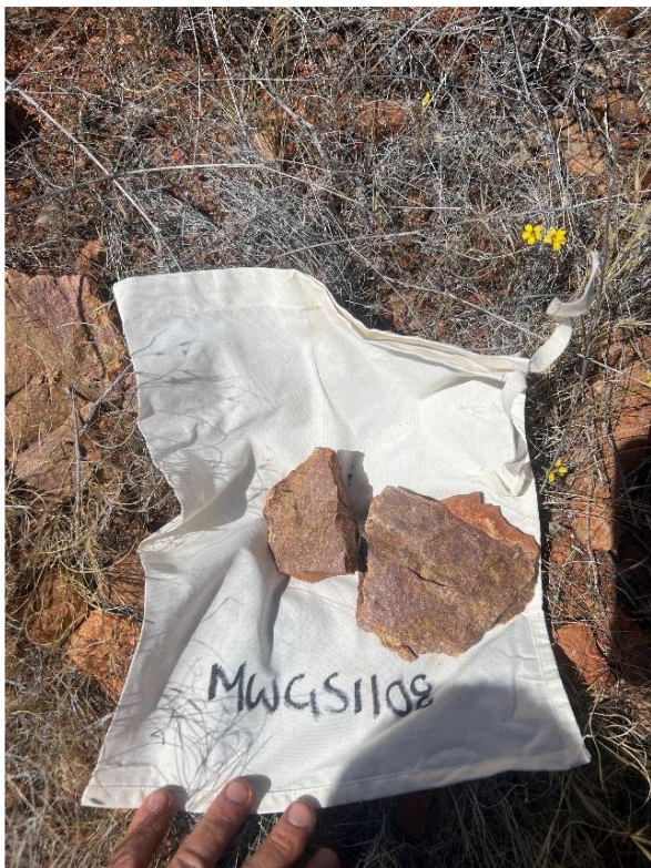
Figure 2: Massive monazite sample MWGS1108 (left) and MWGS0848 (right) which assayed 28.07% TREO with 4.63% \text{Nd}_2\text{O}_3 + \text{Pr}_6\text{O}_{11} and 23.81% TREO with 3.97% \text{Nd}_2\text{O}_3 + \text{Pr}_6\text{O}_{11} .
