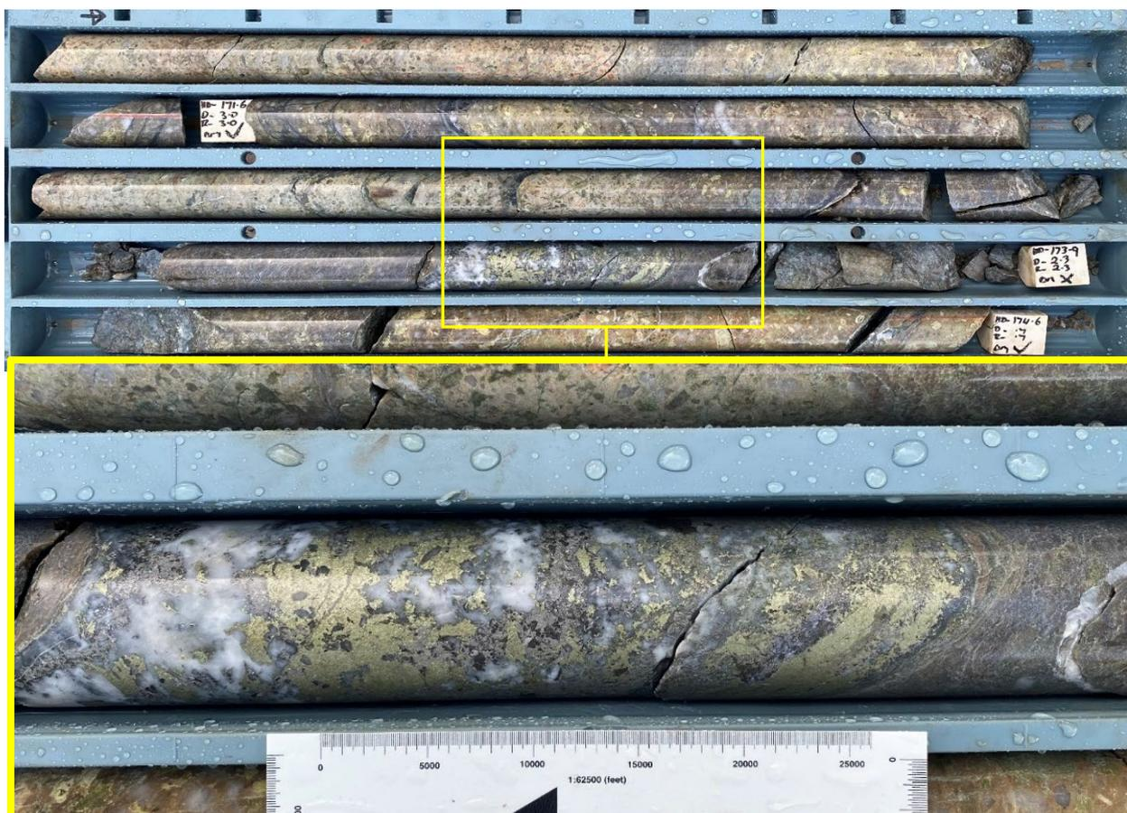
Figure 6 - From mineralised zone returning 19m @ 0.3 g/t Au from 171m *incl.* 1m @ 3.5 g/t Au from 181m & *incl.* 1m @ 3.0% Cu from 173m (22NGD108)
