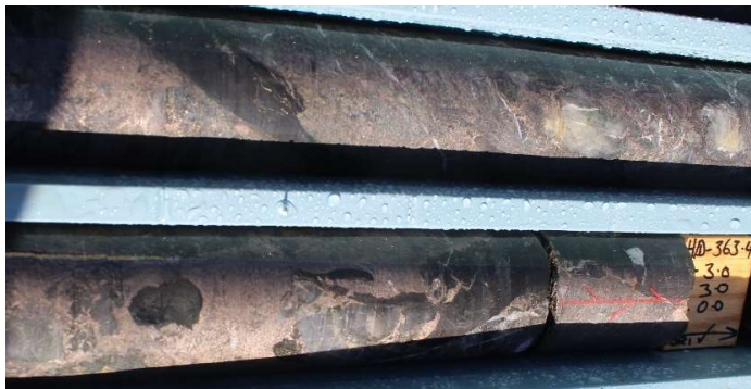
Photo 1: Massive/matrix breccia sulphides, 363m.
