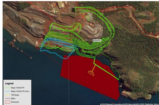
Switch Pit - Concept design highlighting key infrastructure and barge loading location
