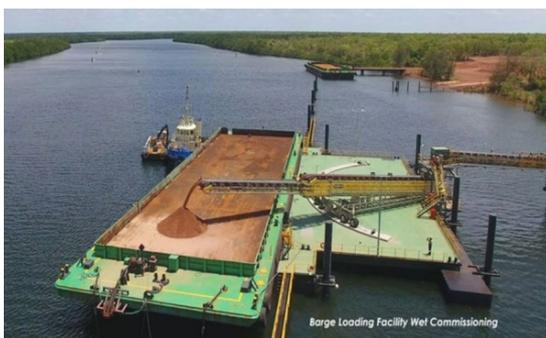
Example of barge loading using a pontoon mounted radial stacker. A similar concept has been proposed for Cockatoo Island
