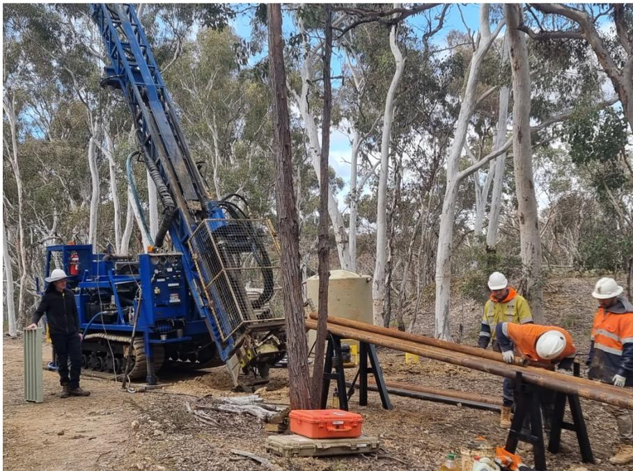
**Figure 1 Diamond rig drilling at Red Hill**
