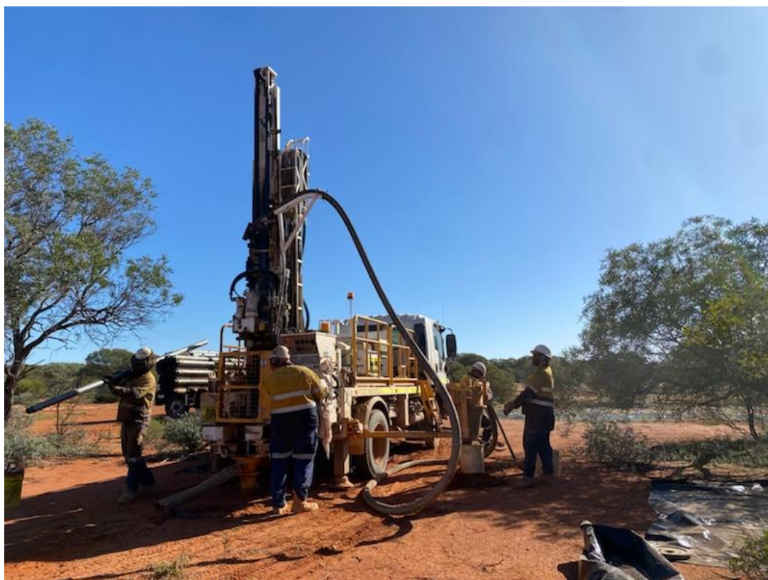
Figure 2 - Photo of Seismic Drilling AC drill rig completing the final hole at North Stanmore E 20/871.
