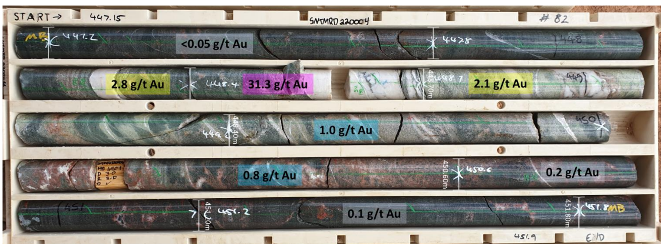
Figure 11 - SN_TM_RD_22_0004: 447.15m to 451.9m Mineralised veins in mafic contact zone western hanging wall to tonalite.
