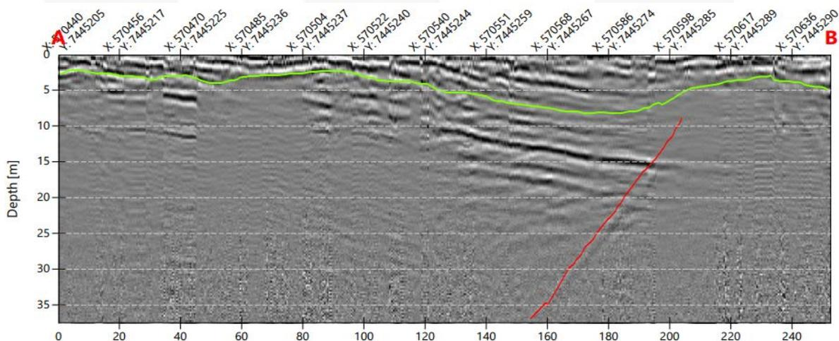
**Figure 9: GPR Profile Target P\_3, interpreted base of alluvium shown in green**
