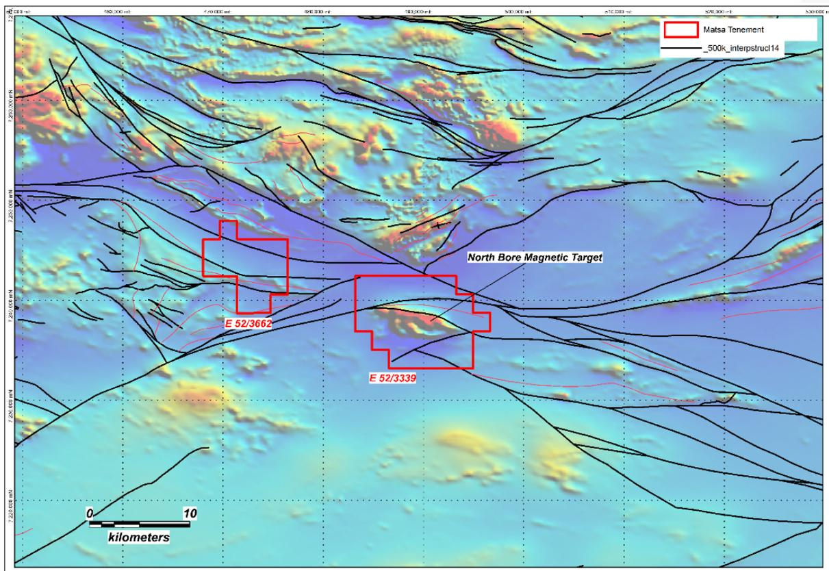
**Figure 10: Location of North Bore project on aeromagnetic image and summary of major faults**
