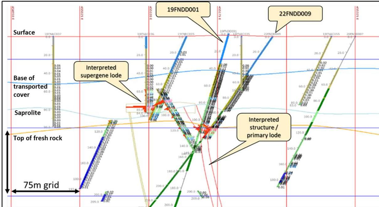
**Figure 4: Fortitude North cross section with new drill hole 22FNDD009**
