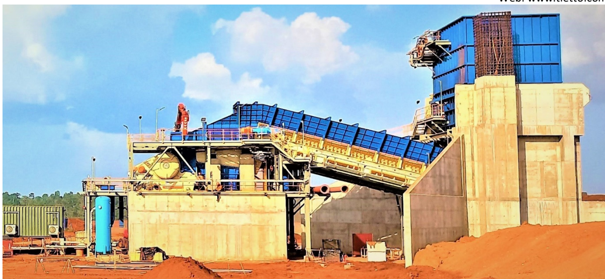
Figure 4: Crusher and ROM Bin installed
