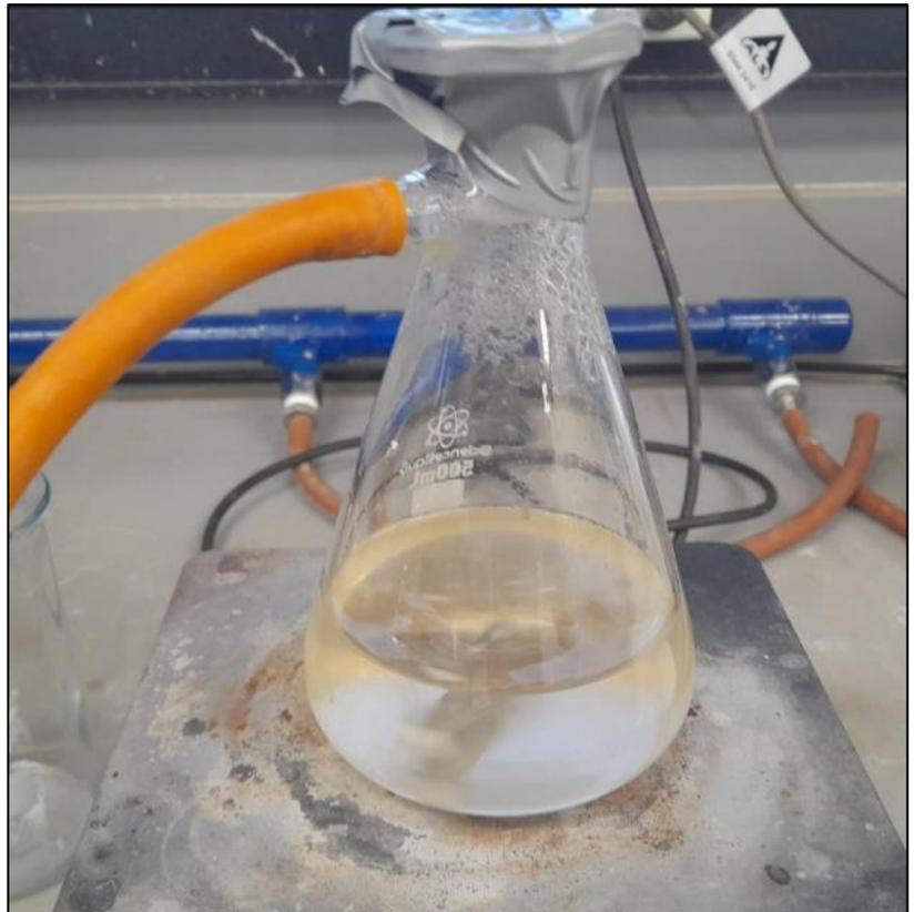
*Figure 2. Mn leachate from the initial test work completed using manganese oxide ore*
